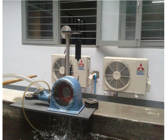
Fig.5. Laboratory scale of model 12 Pelton turbine.
